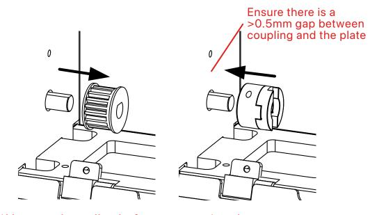
\*Heat up the pulley before unscrewing the set screw
